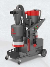
Motor: 5.5 kW / 7.5 hp Power: 3×480 V / 3×240 V FLA: 11 Amp / 23 Amp Weight: 494 lbs CFM: 353 Vacuum: 35 kPa
