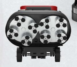
Motor: 2×22 kW / 2×30 hp Power: 3×480 V FLA: 90 Amp Weight W/O vacuum: 3,826 lbs Weight of grinding head: 1,667 lbs Grinding pressure: 2,160 lbs
