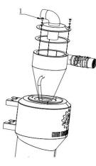
Remove the cover from the integrated bucket, remove the suction hose from the cyclone, illuminate it with a flashlight, check if the inside is blocked, and clean the inside of the cyclone if necessary.
